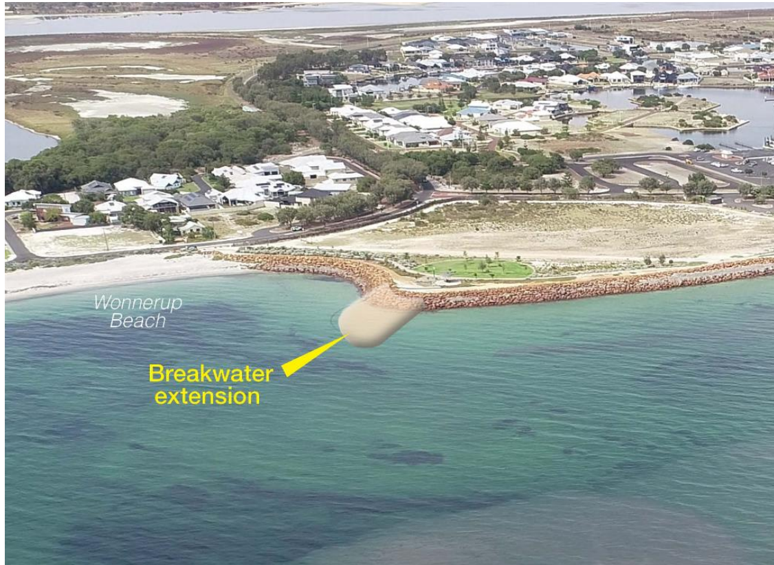
Figure 35: Idea Wonnerup 8 – Extend Eastern Revetment Nib
