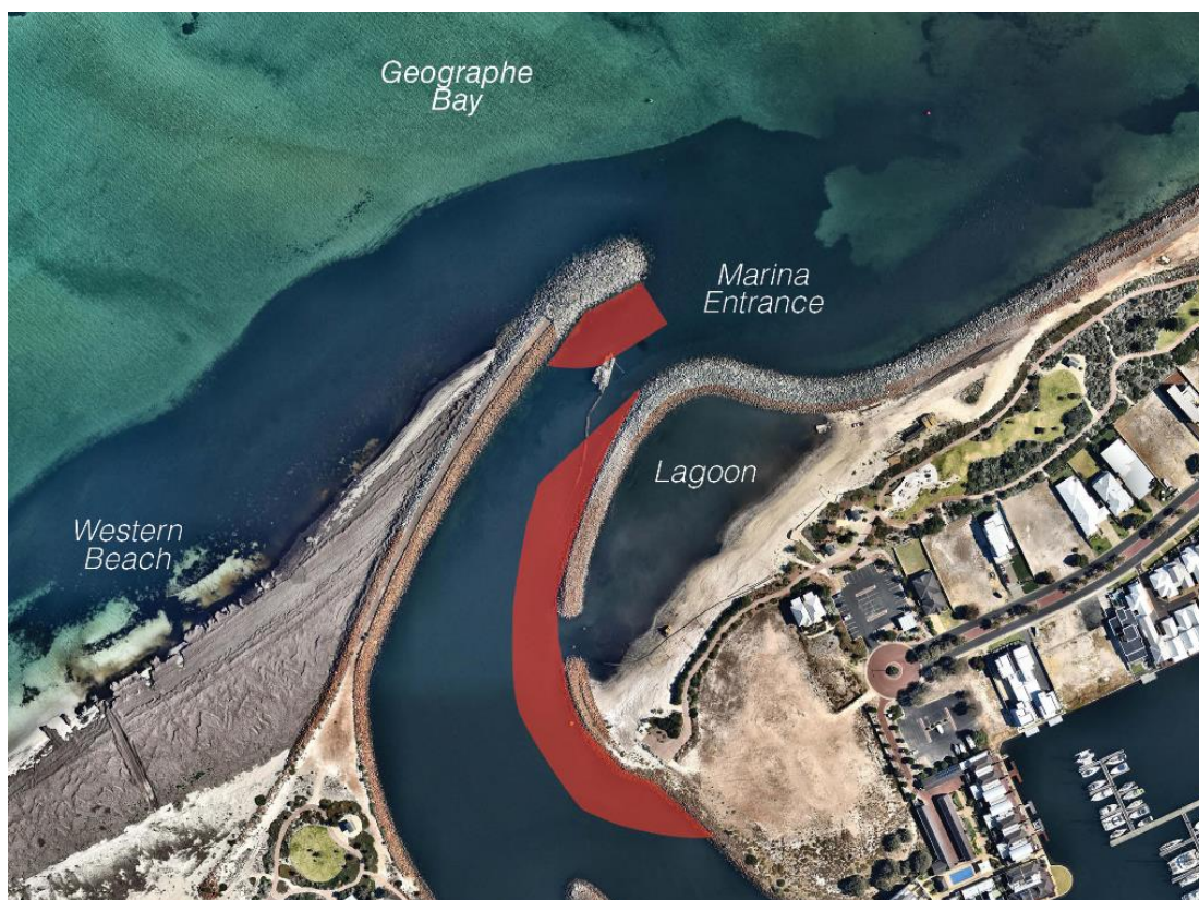
Figure 41: Idea Channel 2 – Reduce dredging to central section leaving narrower channel
