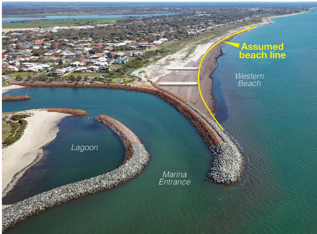
Figure 19: Western Beach 4 – Right-Angle Low-Profile Sand Bag Groynes
